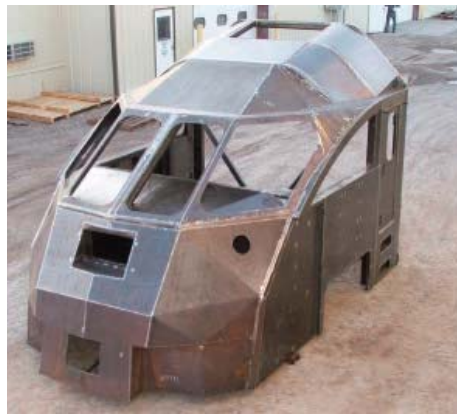
FIGURE 2 This train cab must be fabricated to precision tolerances, with certain large elements needing to be positioned to within 1/16 in.
