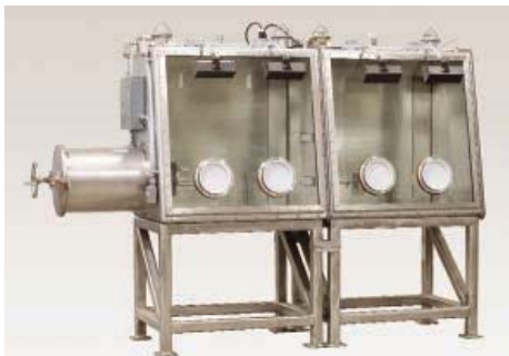
FIGURE 1 Diversified Metal Products fabricated this glovebox for use in the nuclear industry.
